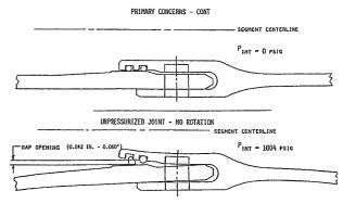
PRESSURIZED JOINT - ROTATION EFFECT (EXAGGERATED)
